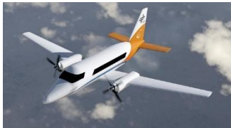
CoCoRe Projekt Hybrid-electric commuter High battery utilization
