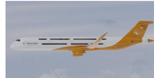
LH 2 wide-body aircraft Liquid hydrogen Gas turbines, fuel cell hybrid options
