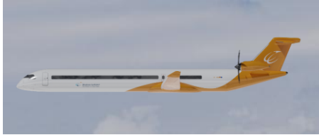
LH 2 Regional Aircraft Liquid hydrogen Fuel cells / propellers
