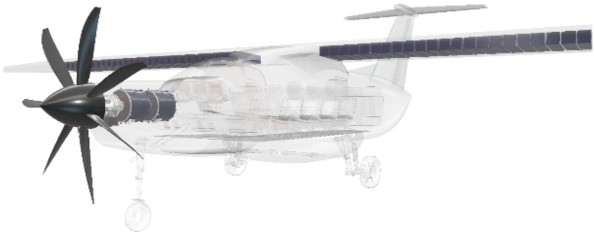
The Microliner benefits from its innovative aerodynamic design: its wing-integrated battery architecture optimizes structural weight and maximizes range. Combined with a novel powerplant architecture, it delivers tangible energy efficiency without compromising safety or passenger comfort. Proprietary technology patents further protect these innovations, reinforcing the company’s role as a trailblazer in zero-emission commercial aviation solutions.
