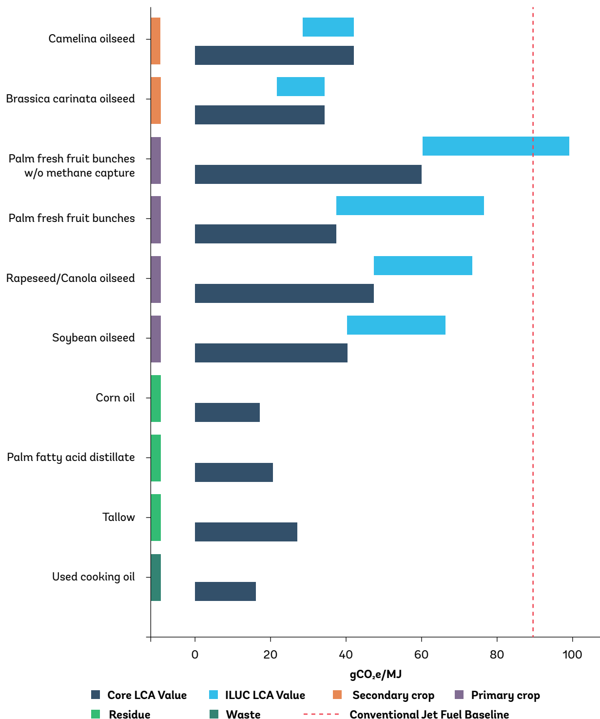
Figure 4A.1 Default lifecycle emissions within CORSIA for SAF produced from oily feedstocks
