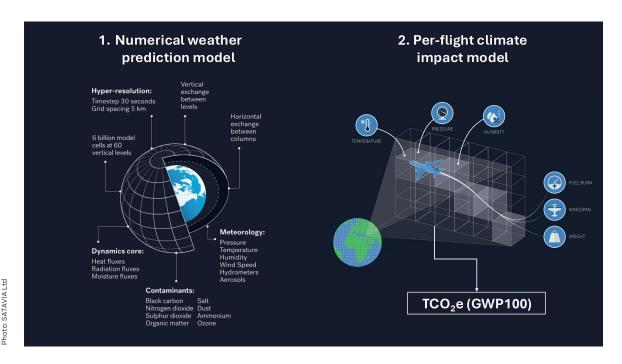
The model is configured for the prediction of relative humidity and other key parameters at cruise altitudes, with enhanced vertical resolution alongside explicit physics-based cloud microphysics. These NWP enhancements are necessary, as off-the-shelf weather models show strong dry bias at cruise altitude, increasing the probability of false negative predictions of contrail-forming conditions and potentially allowing flight into seemingly dry atmosphere that may, in reality, be supersaturated.
